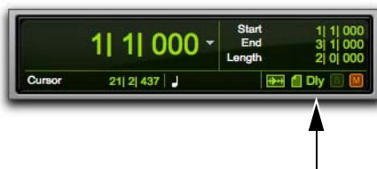
Delay Compensation indicator
