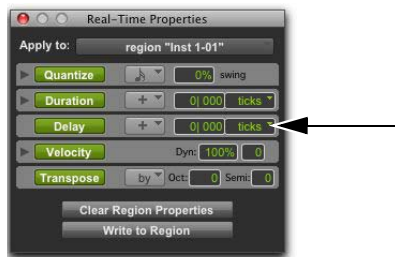
Real-Time Properties Ticks/Milliseconds pop-up menus
