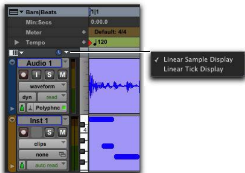
Linearity Display Mode selector and pop-up menu
