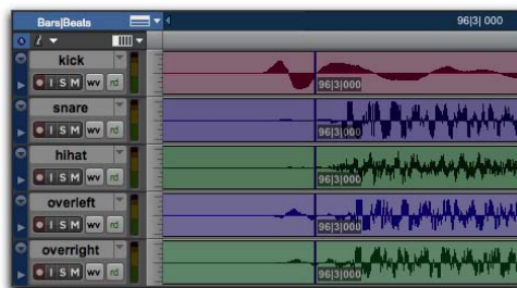
Overhead mics generate late beat triggers
