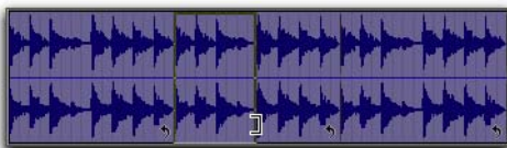
Trimming a looped clip
