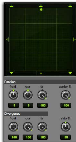
Side % set to 50% (side center speakers dimmed)
