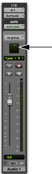
Drag to pan in the Track Grid
