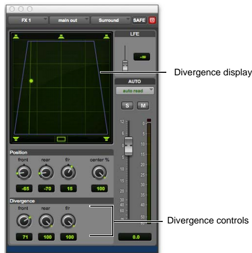
Divergence display and controls
