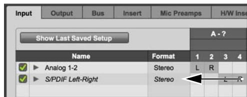
Unavailable hardware Input shown in italics
