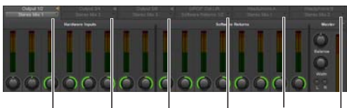
Tabs representing each Mbox Pro hardware output pair, output pair select view shown
