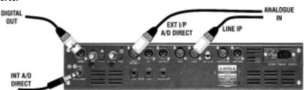
The optional A/D card is a stereo device which can convert two tracks simultaneously. Stereo conversion can be accessed by connecting the two audio signals into the EXT A/D DIRECT and INT A/D DIRECT inputs (directly accessing the A/D inputs via the limiter and digital meters). The INT input of the A/D can also be connected in the normal way via the Line I/P, if additional mono processing (EQ and Dynamics) were required on the signal, or if dual mono signals were being converted simultaneously.
