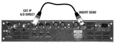
This example shows the insert send feeding the "External I/P A/D Direct" input. This allows an analogue input to be connected to the insert return, and then routed, via the dynamics modules, to the digital output.
